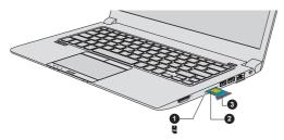
Figure 4-8 Installing the SIM Card (Z40-A)
